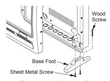
Figure 13 - Installing Base Feet
